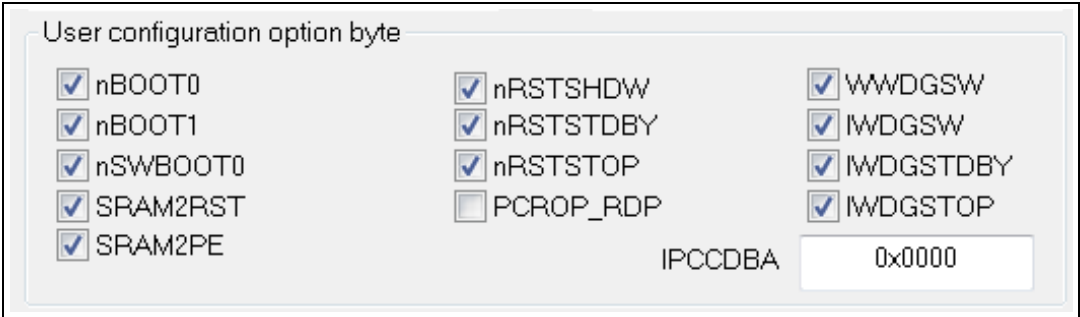
Figure 54. Option bytes configuration for MAC 802.15.4
